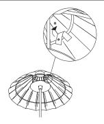
3. Attach the leather shade to the frame using the three leather straps with press studs.
