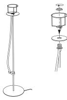
2. Assemble the parts on the lampholder as shown in the figure above.
