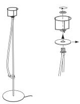
For a greater light output, remove the round metal plate.
